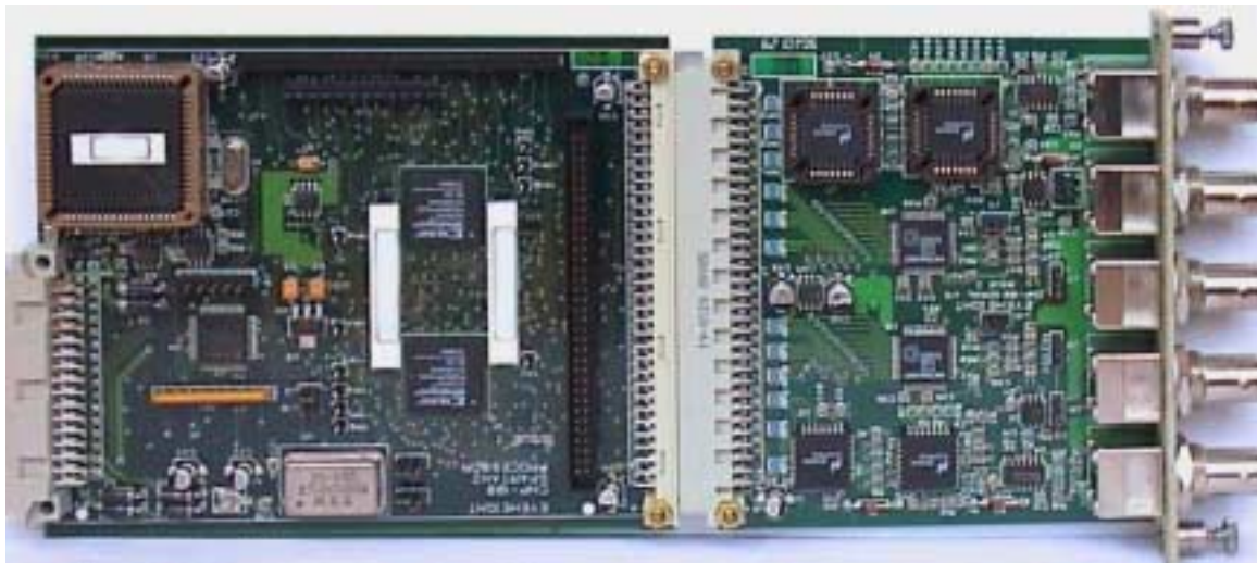
Figure 1-1 The SA-1 safe area generator PCB.
