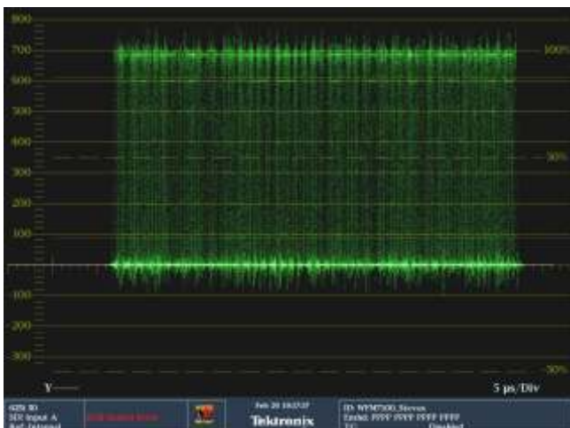
A typical title produced in Motion legalised using the built-in "Broadcast Safe" filter.
